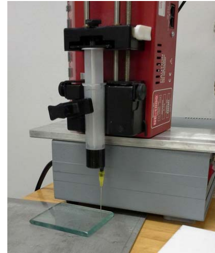
Figure 7-1 Test apparatus including the programmable syringe pump
