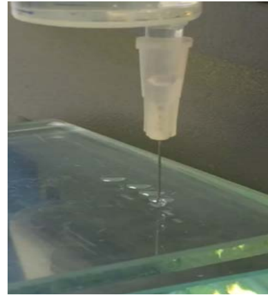
Figure 7-2 Extrusion test of the pure polymer precursor
