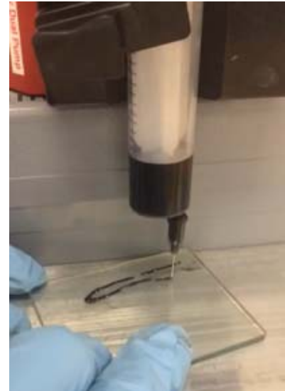
Figure 7-6 Syringe loaded with CNT mixture
